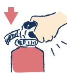
4 Squeezing the lever releases the fire extinguishing agent from the nozzle.
