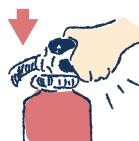
Squeezing the lever releases the fire extinguishing agent from the nozzle.
