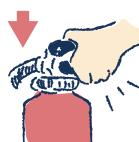
4 Squeezing the lever releases the fire extinguishing agent from the nozzle.
