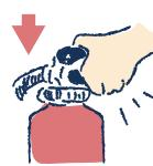
Squeezing the lever releases the fire extinguishing agent from the nozzle.
