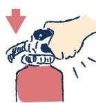
4 Squeezing the lever releases the fire extinguishing agent from the nozzle.
