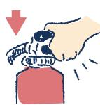
Squeezing the lever releases the fire extinguishing agent from the nozzle.
