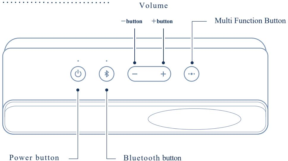
1. Press the power button
